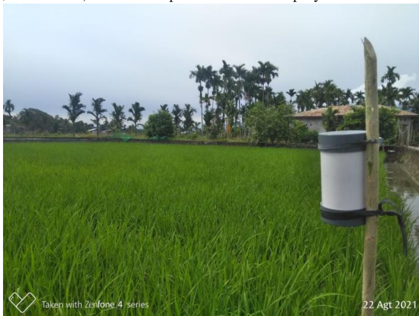
Figure 4. Application of automatic bird repellent in paddy fields
